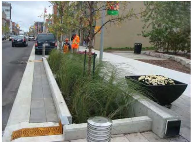
Vegetated curb extensions can be installed where pavement width can be reduced along segments of a street. These curb extensions can be placed where no parking areas already exist, such as near intersections. They can be combined with bulb-out curbs to reduce the width of street that must be crossed by pedestrians.
